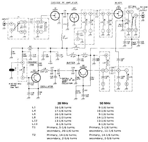
fig. 5. Whf converter for use on the six- and ten-meter amateur bands. All inductors and transformers wound with no. 26 (0.4mm) wire.
